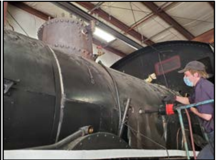
No. 9 is stripped to allow the cleaning and testing of the boiler. These pieces of equipment are in storage until the boiler work is complete.
