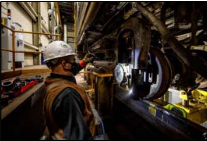
Removal of the old wheel and replacement process with new wheel in 6111's truck.
