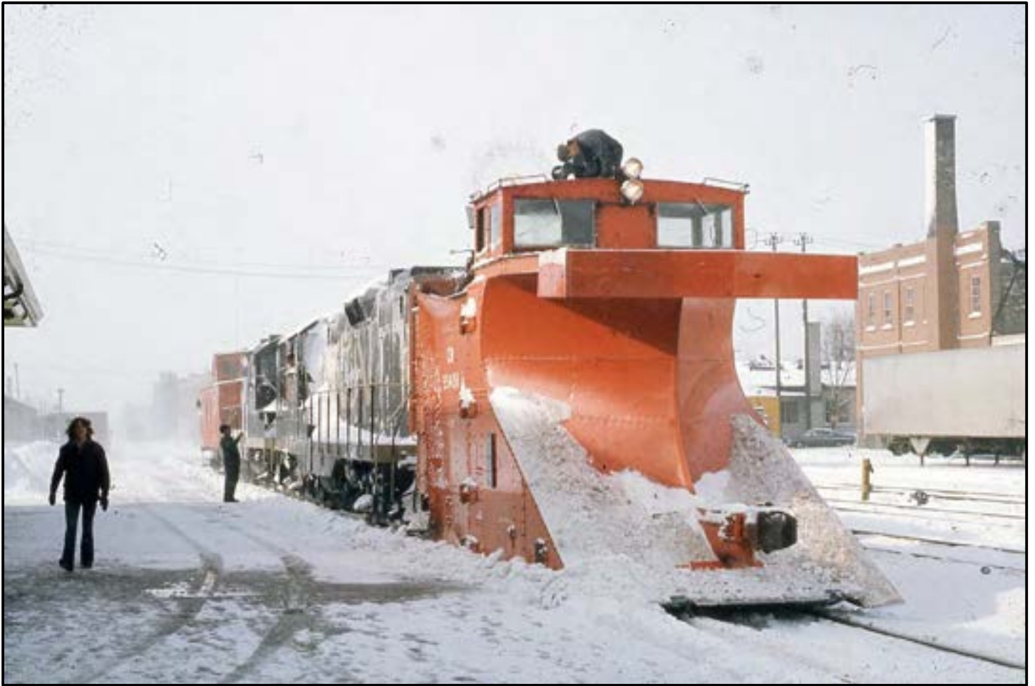
In February of 1972 CN plow extra heading west and then ultimately to Elmira sits at the Kitchener Station while the Plow Foreman works on the plow cupola roof to free snow from the air horns.
