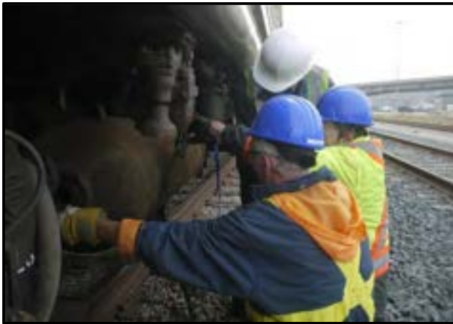
Borrowed air brake reservoir is installed in 6111 to replace one that had been removed over the years.
