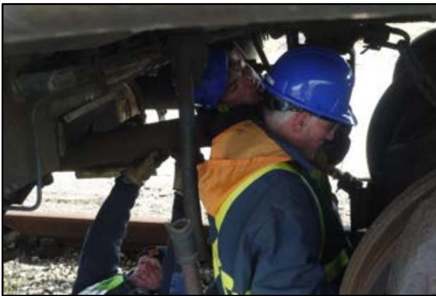
Each RDC unit has a direct drive shaft from the diesel engine slung underneath to one axle per truck assembly.
