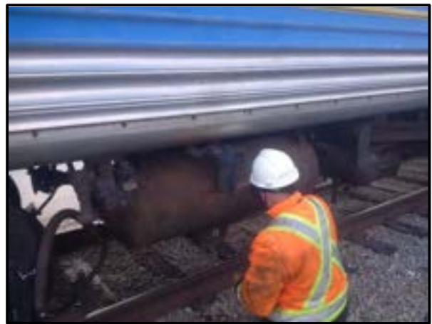
Borrowed air brake reservoir is installed in 6111 to replace one that had been removed over the years.
