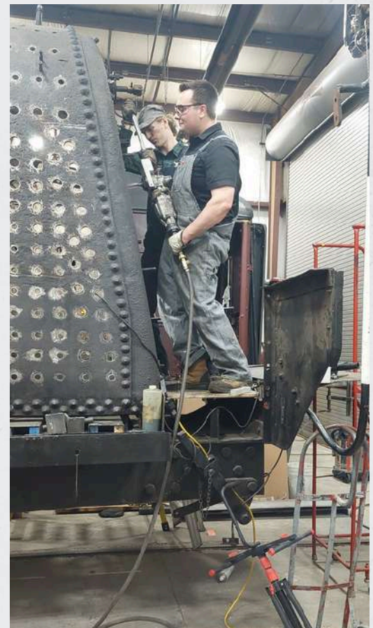
Jake & Andrew drilling staybolt holes
